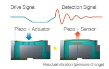
Ensure consistent, uninterrupted quality with Nozzle Verification Technology that detects blocked nozzles, and dot compensation that compensates for them.
